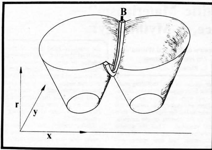
Figure 3. The space of possible configurations of the wheel (b) in Figure 2. The thin strip B represents the configurations in which wheel (b) meshes with both (a) and (c).
